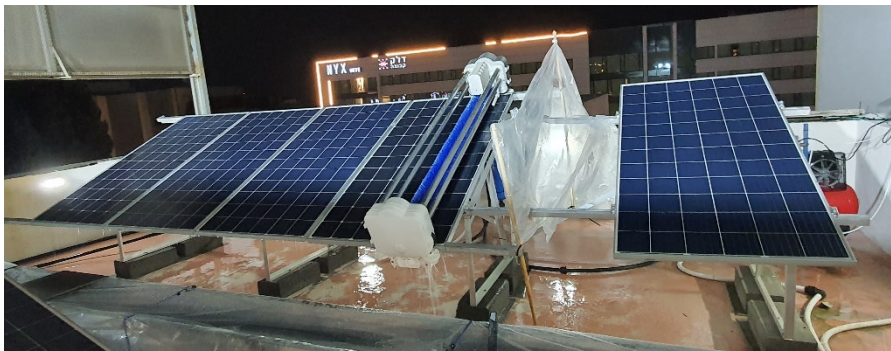
Figure 4-2: Test setup, cleaning robot in parking position and test modules mounted. The left and right modules of this group of four are the parking positions for the robot. The test modules are the two middle ones.
